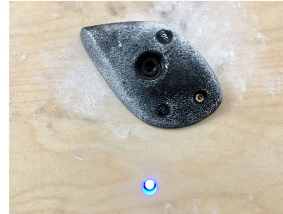
An intermediate hold lit by a blue LED, indicating its use on a problem.
